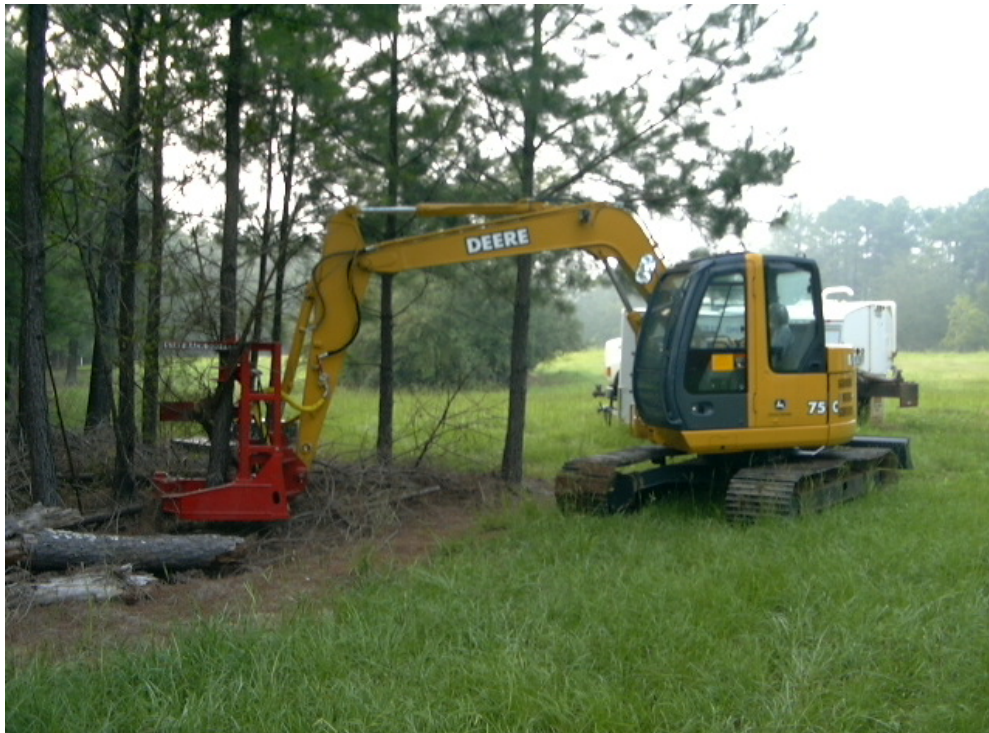
Figure 1. John Deere 75C with a Fecon shear head.
