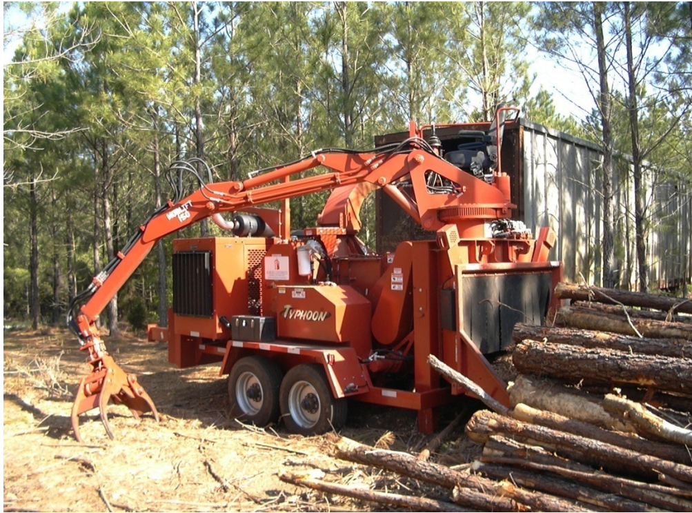
Figure 3. Morbark Typhoon chipper with a loader attachment.
