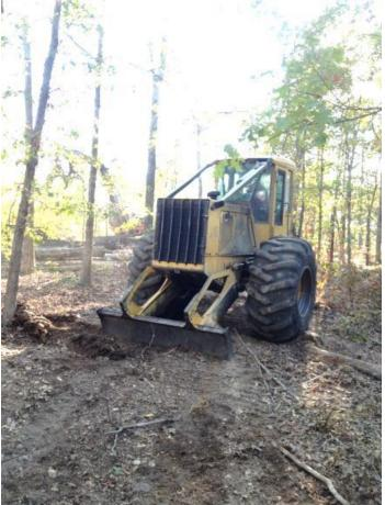
The skidder will need to reposition and push a minimum of four different times to correctly complete the construction of a waterbar. Pictured here is the second push.
