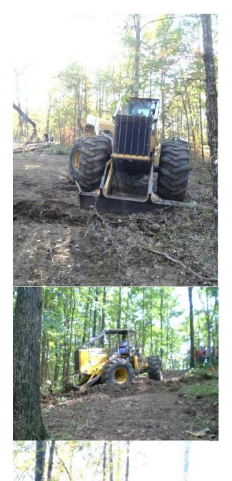
The skidder is currently completing the third push. Notice that the waterbar extends beyond the lower end of the skid trail preventing water from running back into the skid trail.
